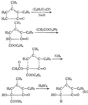
The final product (Ic) distilled at  $92^{\circ}$  (0.3 mm.);  $n^{27}$ D 1.4930.
